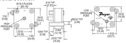
Series MDA Miniature Adjustable Pressure Switch is used to sense differential pressure. The switch features field adjustable set point and gold inlay contacts. Air or other compatible fluids can be used on the "high side". The lightweight and compact size make the MDA ideal for any application with space constraints. Applications include industrial, HVAC, pump and motor control, medical, automotive, pools and spas.
