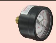
The Series UGI Utility Gages possess dual psi and bar (x100 kPa) scales with  $\pm 2.5\%$  accuracy. The UGI gages are designed with black steel housings. Wetted parts include a brass socket and phosphor bronze tube. A wide offering of ranges are available from full vacuum to 300 psi. The center back mounting and compact size makes this gage the perfect choice for pneumatic air regulators.
