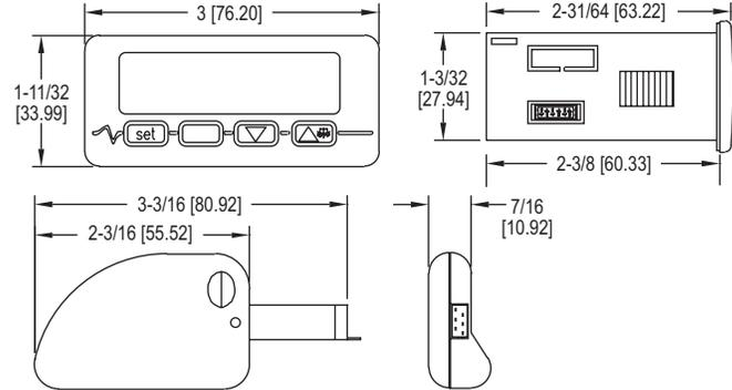
The Series 40T/40M Digital Temperature Switch accepts a variety of inputs to allow temperature measurements and set points up to 1999°F (1300°C).
