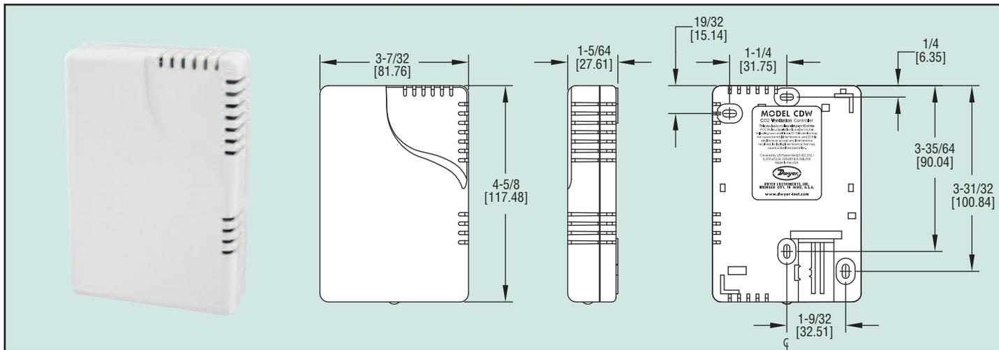
The Series CDW Wall Mount Carbon Dioxide/Temperature Transmitter combines accurate CO<sub>2</sub> measurements with a passive temperature output. The Non-Dispersive Infrared (NDIR) sensor continuously updates the calibration through a proprietary logic feature which limits the amount of error due to drift. The CDW series is ideal for building automation systems to help control the fresh air intake in a room.
