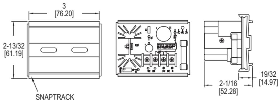
The **Model BPS-005 Low Cost DC Power Supply** is a regulated .5 A power supply that accepts 24 VAC input and provides an adjustable 1.5-29 VDC output. Output voltage adjustments are made using the on-board potentiometer while measuring the output with a multimeter. A compact snap track design allows the power supply to be surface mounted within a panel.
